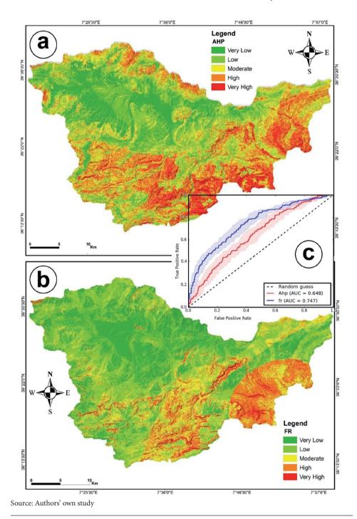
Fig. 4. a. Landslide susceptibility map derived from the AHP model. b. Landslide susceptibility map derived from the FR model. c. AUC validation of Ahp and FR models
