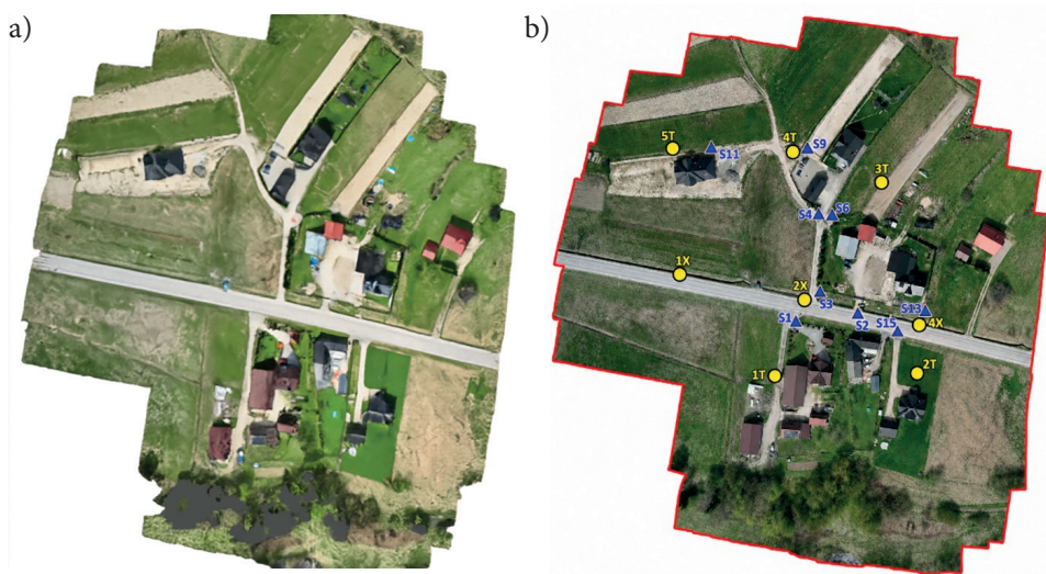
Fig. 4. Photogrammetric data processing results: a) dense point cloud and b) spatial distribution of ground control points (circles) and independent checkpoints (triangles) within the study boundary
