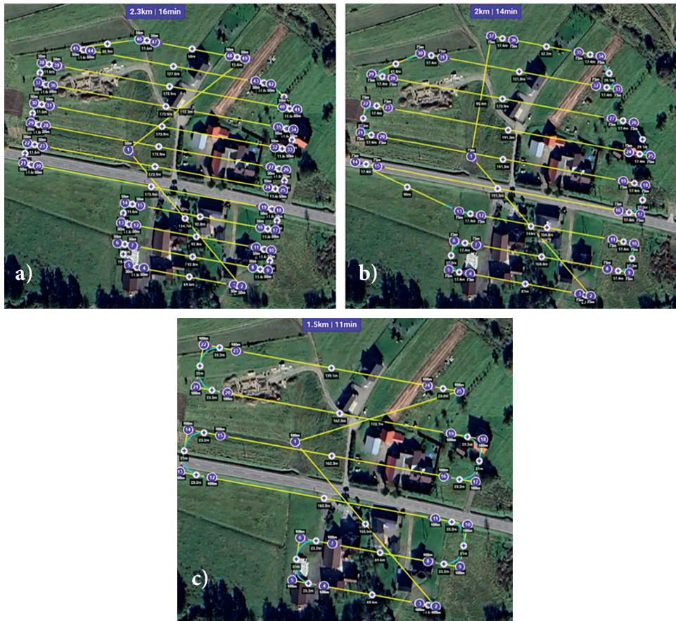
Fig. 3. Flight mission plans developed in the Litchi Pilot application for flight altitudes of: a) 50 m - planned route length of 2.3 km and estimated flight time of 16 min; b) 75 m - 2.0 km and 14 min; and c) 100 m - 1.5 km and 11 min.
