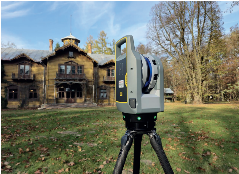
Fig. 3. Trimble X9 laser scanner used during field measurements
