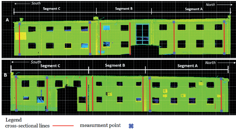
Fig. 3. East elevation (A) and west elevation (B) – point cloud with designed profiles marked by red lines
