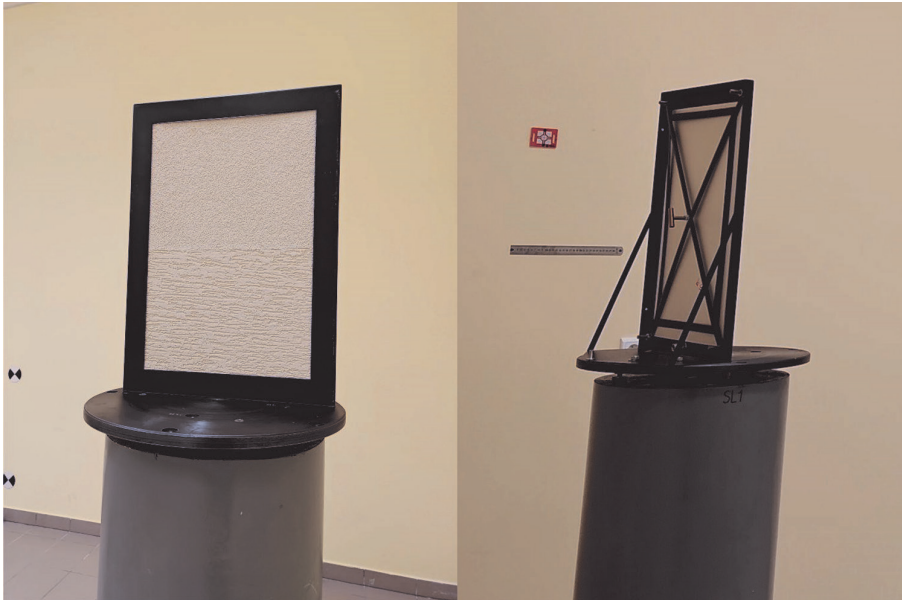
Fig. 3. Measuring frame for positioning the plates during measurement
