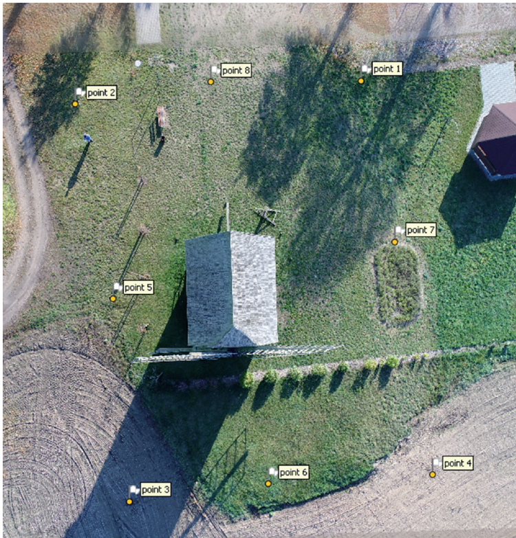
Fig. 3. Ground control points and check points used in the aerotriangulation process
