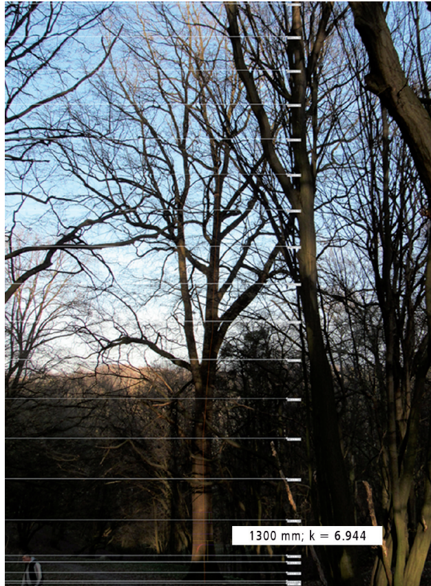
Fig. 7. Image of the plane of the tree trunk survey with the height levels marking. The callout shows the height of the level and the parameter k . Such indicators are given at all levels of the horizon
