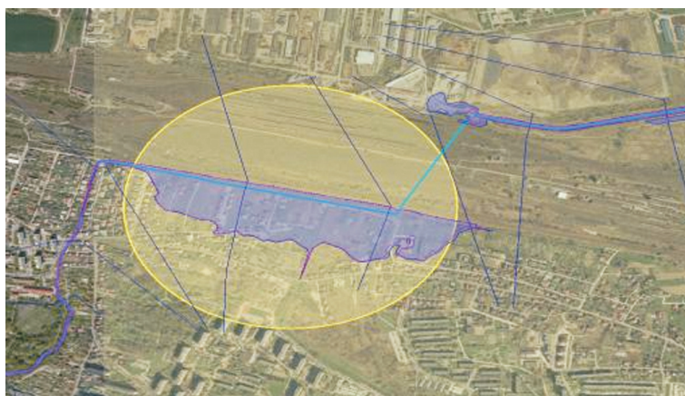
Fig. 7. The danger zone on the river Drwinka due to the culvert obstruction
