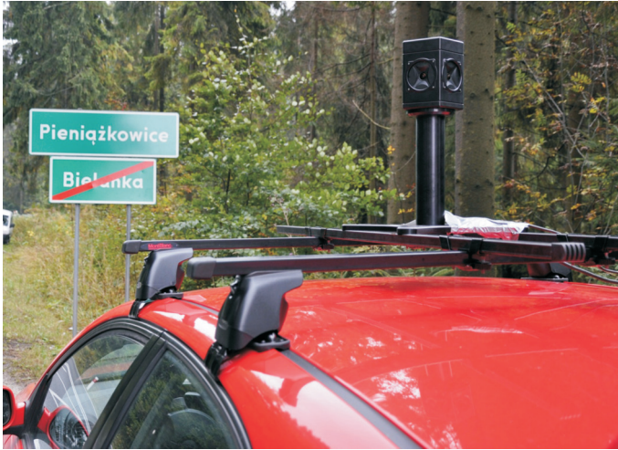
Fig. 9. Ladybug© 3 camera installed at the top of the car before recording the district of Czarny Dunajec in Poland
