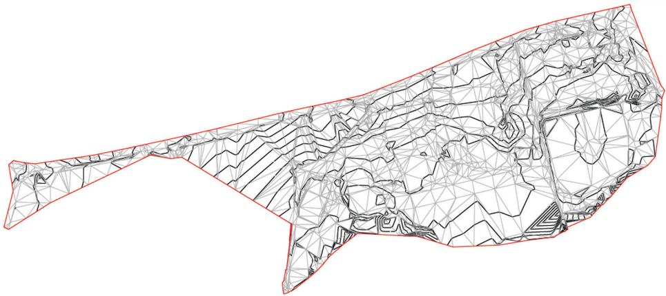
Fig. 2. Output data: network triangles supplemented with contour lines
