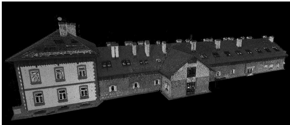
Fig. 1. Processed point cloud of a teaching facility at the University of Agriculture in Krakow
