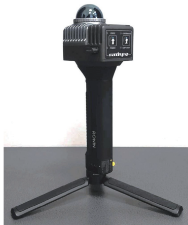
Fig. 3. MandEye LIVOX MID-360 mobile laser scanner
