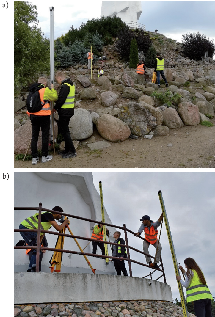
Fig. 1. Measuring vertical displacements: a) view of the mound, b) approach to the base (pedestal) of the statue
