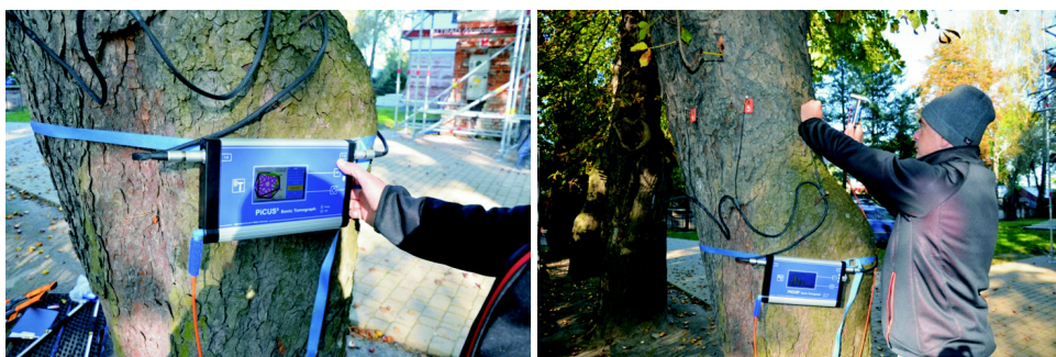
Photo 1. Central unit of the Picus 3 ultrasound computed tomography device (photo by M. Dudkiewicz, 2017)
