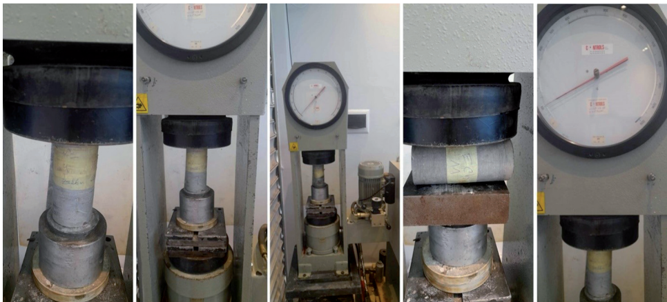
Fig. 6. Mechanical test for uniaxial compression strength performed with a uniaxial compression press
