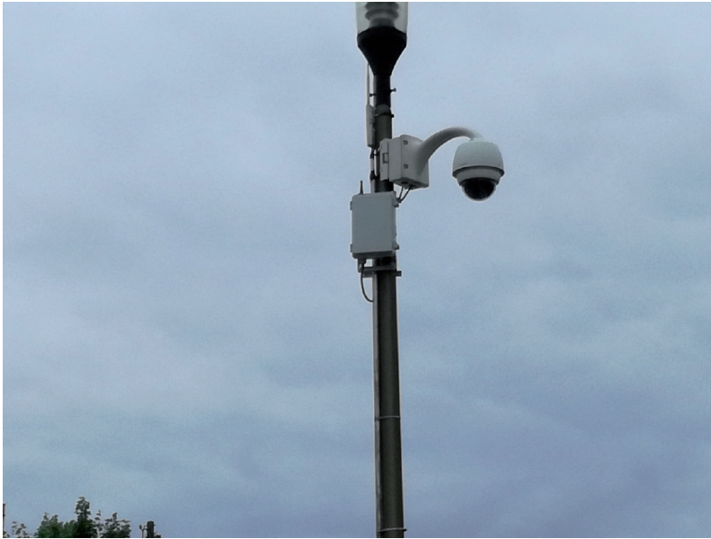
Fig. 7. Sensor network coordinator and edge server
