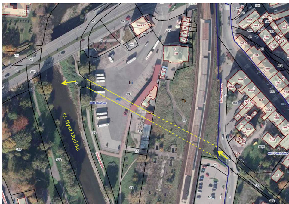
Fig. 2. Procedure of determining boundaries of land plots at the street of al. 29 Listopada
