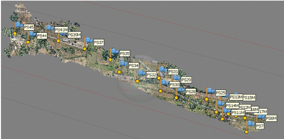
Fig. 3. Location of all the points of the geodetic control network in the model
