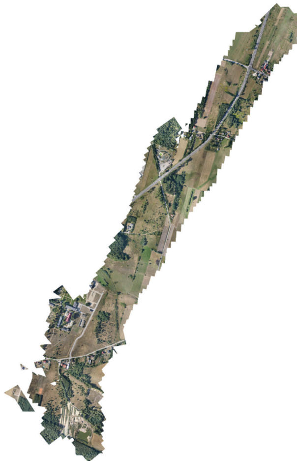
Fig. 5. Orthophotomap developed based on an UAV mission flight
