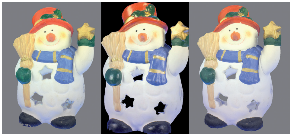
Fig. 6. a) Left: model executed without the colour calibration; b) Middle: image after the calibration and the automatic separation of the background; c) a 3D model executed based on the colour-calibrated images
