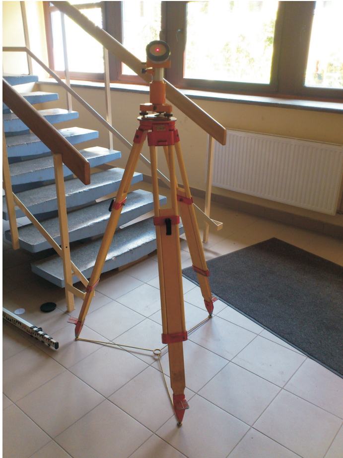
Fig. 6. The plane mirror station on a geodetic tripod set at the ground floor of the studied building
