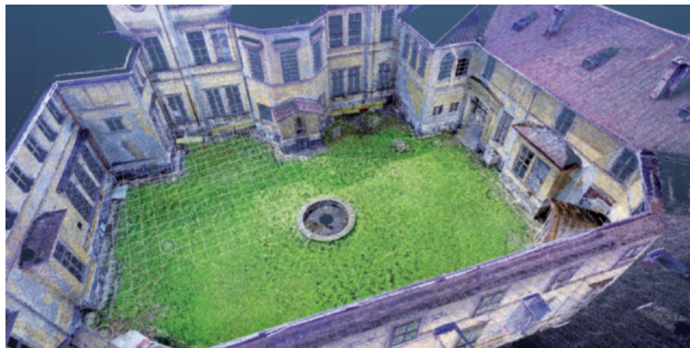
Fig. 7. View of the palace as a coloured point cloud
